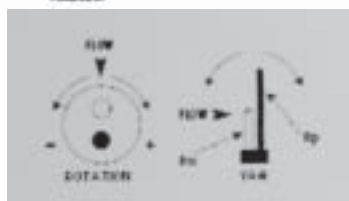
Figura 5 Sensor Rotation and Yaw Alignments
